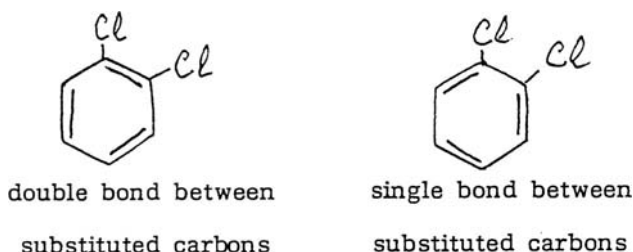
Figure 4: Two classic representations for 1,2-dichlorobenzene, one with a single bond the other with a double bond between the substituted carbons. The actual molecule has a bond intermediate between single and double.
